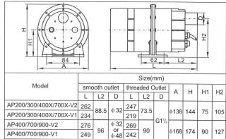
1. D in fig.is thread connection that union of  $\varphi$  32and  $\,\varphi$  33.5 available 2. D in fig.is direct connection that have  $\varphi$  32 ;  $\varphi$  33.5 and  $\varphi$  48 available.
