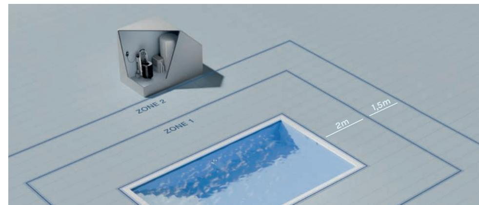
Even though charging the EVAsream Move while in or near the water is strictly prohibited (the unit must be at a distance of at least 3.5m, outside of pool zone 2), the PRCD switch is an extra safety measure to minimize the risk of electric shock resulting from (unintentional) water contact.
