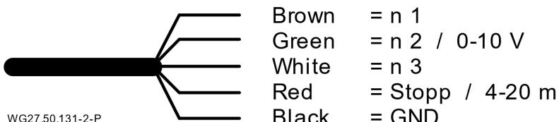
The cables must be connected potential free. Only switch the contacts individually (observe priority of the contacts). Otherwise the desired speed is not activated. The digital inputs must be activated accordingly in the Setup menu for external activation.
