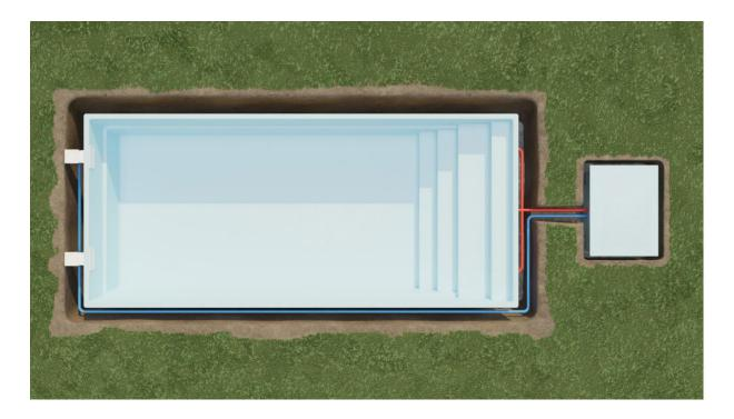
After connecting the devices, we continue backfilling the basin (under the frame) and filling it with water (up to halfway of the skimmer)
