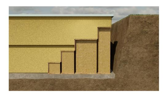
During backfilling of the pool, it is important to observe whether the walls of the pool are bending inward or outward.
