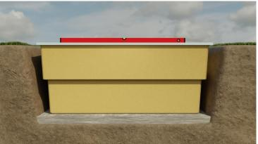
After the pool is set in the excavation, its position in relation to the terrain should be checked.
