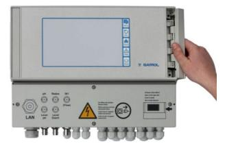
Remove the cover plate and unhook the hinge on the bottom.
