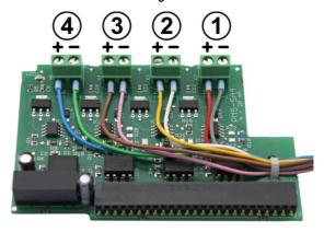
4. Insert the PM5-SA4 plug-in module carefully into the plug-in connector 1 (on the left).
