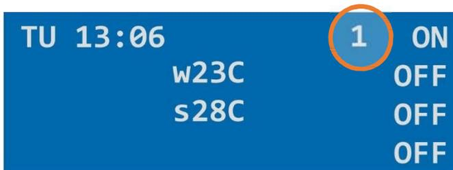
**Figure 2. Display with current values. The 1 in the yellow circle indicates the current pump speed.**
