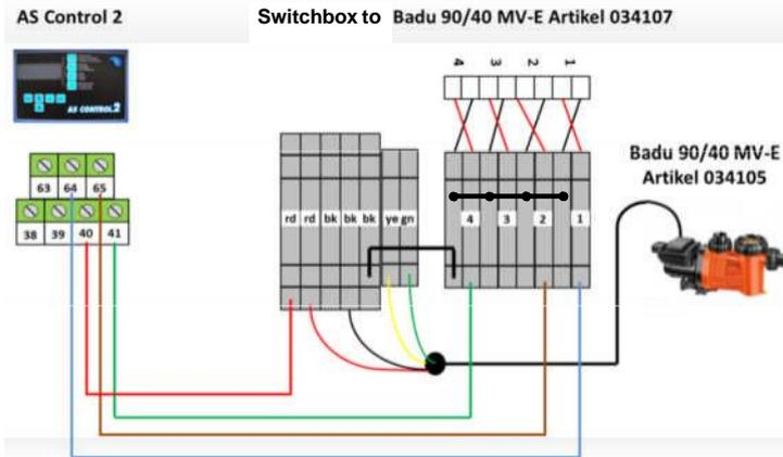
Figure 15. Connecting Speck Badu 90/40 MV-E + Switch box 034107
