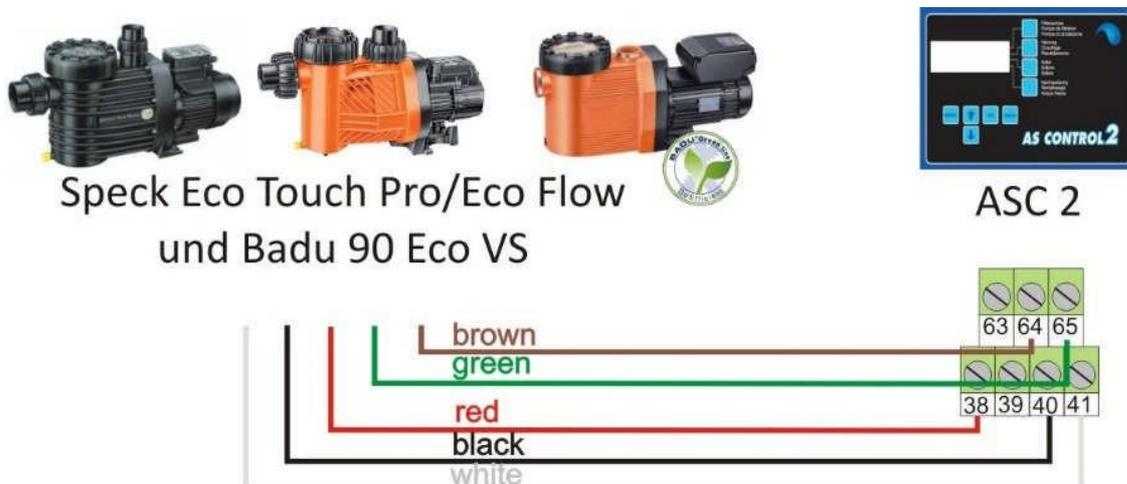
Figure 14. Connection of Speck Eco Touch Pro and Badu 90 Eco VS
