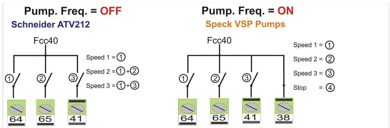
**Figure 12. Function/principle of frequency regulation of Schneider ATV 212 and Speck VSP.**
