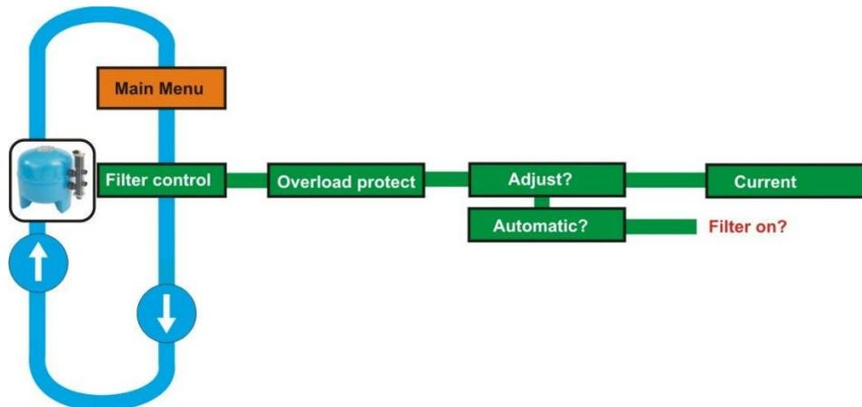
**Figure 9: Setting the motor protection**
