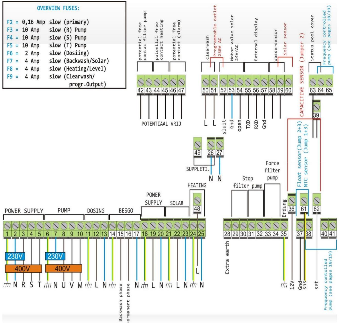
Figure 17. ASC 2 connection terminals
