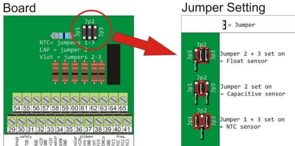
Figure 16. Jumper setting with regard to level regulation/replenishment
