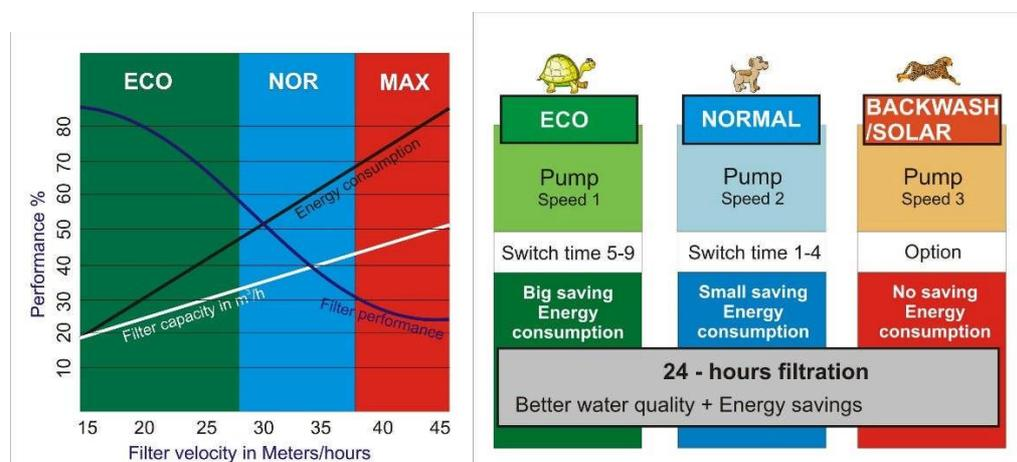
**Figure 7: Filter speed in relation to filter performance and energy costs**
