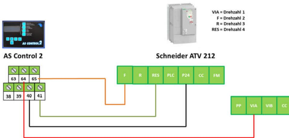
Figure 13. Connection of Schneider ATV 212 Regulator 0.55 kW to 5.5 kW
