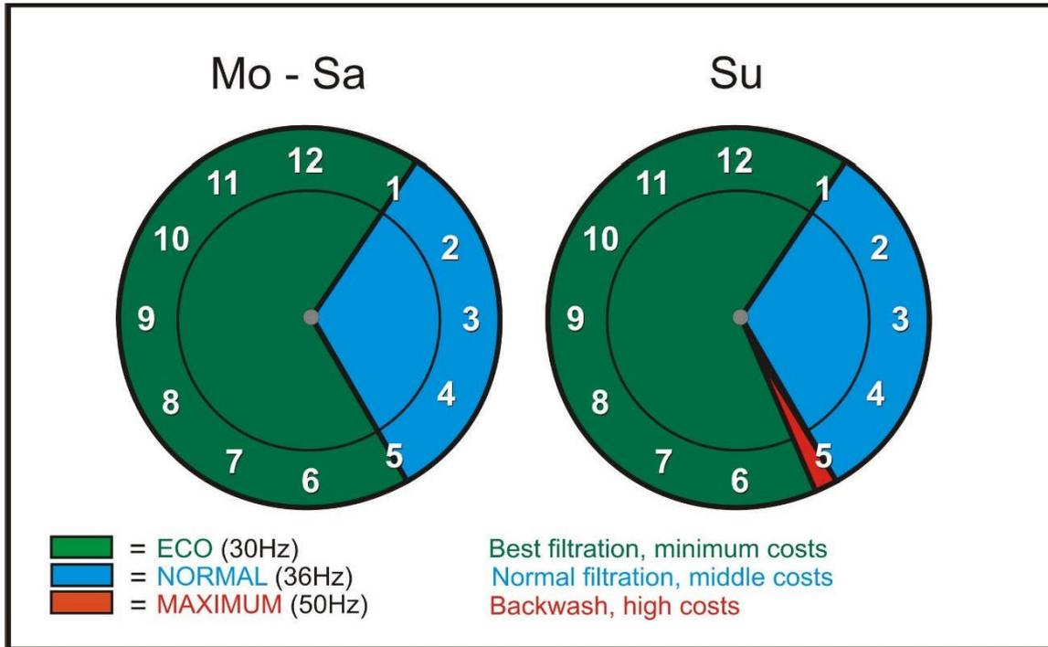
**Figure 8: Example of a weekly programme with 2 filter speeds and a backflush cycle.**
